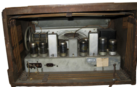
Philco model 42-340T —Two tone wood table radio that covers AM and shortwave bands. Made in 1942 with 7 tubes. Dan Santos, Carlisle, PA
