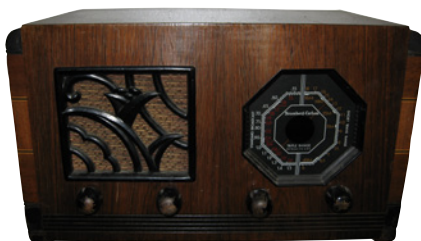
Stromberg Carlson model 225H —Octagonal dial radio covering the AM band. Made in 1937 with 6 tubes. Artie Schwartz, Phoenix, AZ
