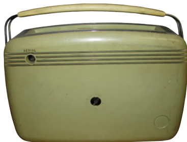
Bush Portable Radio —Model number unknown. This is an English transistor radio that works on a PP9 9 volt battery. Covers medium and longwave bands. Irwin Strongwater, Houston, TX
