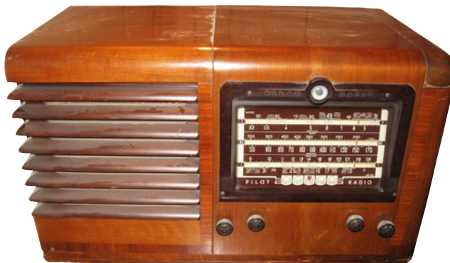
Pilot model 173 —Manufactured in 1941. Large table top radio that covers 3 bands – AM and 2 short wave. John Hewlett, Little Rock, AR.
