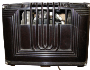
Emerson model BA199 —Bakelite radio made in 1938. Comes with Bakelite back cover, 4 tubes, AC/DC. Alfred Dove, Sioux City, IA.
