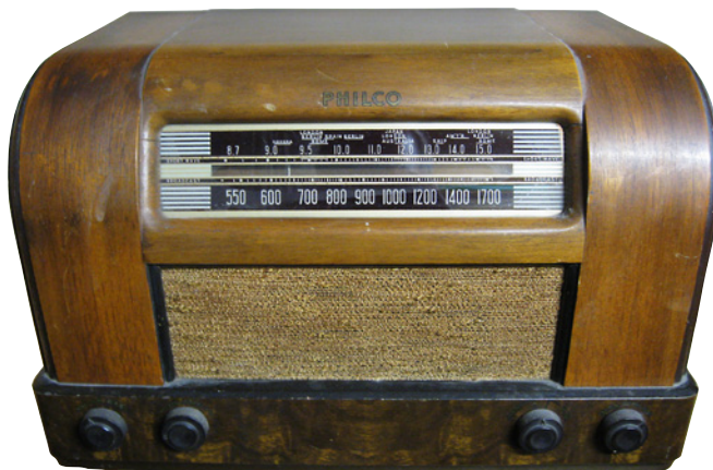
Philco model 42-340T —Two tone wood table radio that covers AM and shortwave bands. Made in 1942 with 7 tubes. Dan Santos, Carlisle, PA
